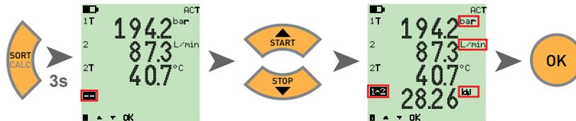
**i** Differential value, addition and power (multiplication) are available as calculating formulas. After the formula has been selected, the measurement variables are checked for plausibility. The error message INERR is displayed if the measurement variables are not plausible.
