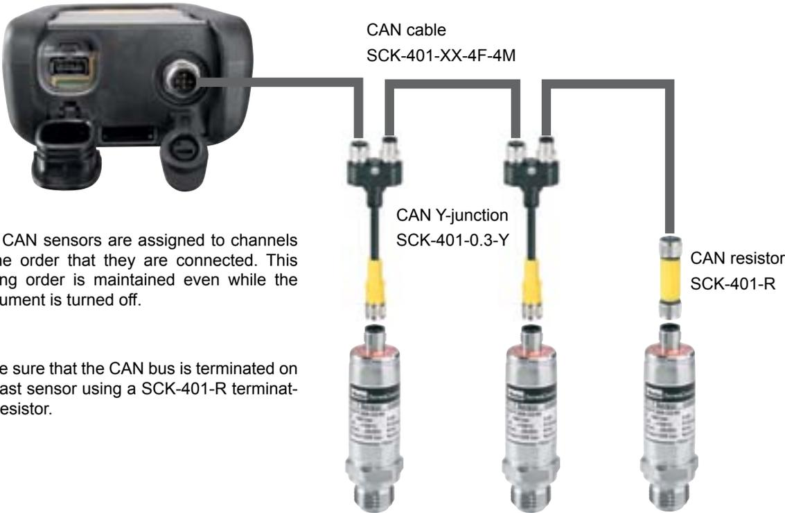
**i** The CAN sensors are assigned to channels in the order that they are connected. This sorting order is maintained even while the instrument is turned off.
